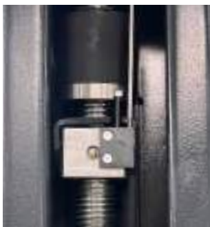
SAFETY SYSTEM to control the wear of the screw and the turning screws
