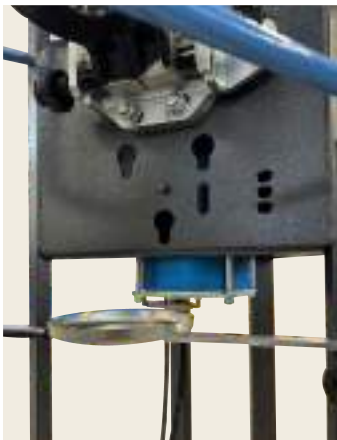
POSSIBILITY OF DOUBLE POSITIONING of the bracket to have more space and stroke for spring compression.
