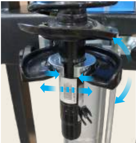
ADJUSTABLE UNIVERSAL BRACKET TO HOLD THE SPRING IN PLACE
