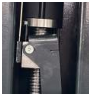
MECHANICAL STOP for automatic locking in the event of a malfunction
