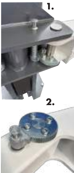
ARM SAFETY LOCKING with automatic engagement and automatic release when the arm reaches the floor
