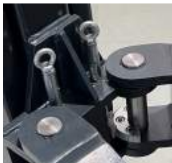
PROTECTION against the possibility of horizontal movement of the arms while the trolleys are raised
