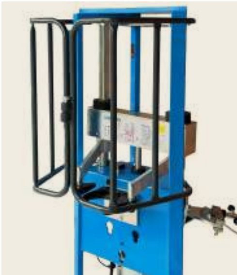
IF THE SAFETY GUARD REMAINS OPEN, THE MACHINE IS EQUIPPED WITH A SAFETY VALVE THAT DOES NOT ALLOW WORKING OPERATIONS
