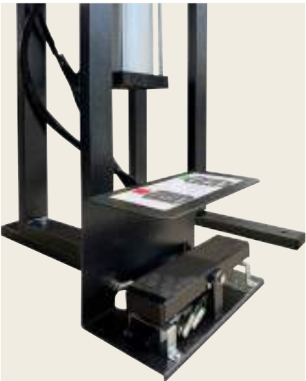
THE FOOT-PEDAL WORKS ONLY WHEN THE SAFETY VALVE IS CLOSED; IF IT IS OPEN THE FOOT-PEDAL IS BLOCKED
