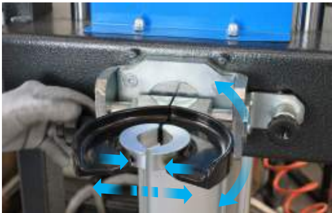
ADJUSTABLE UNIVERSAL BRACKET TO HOLD THE SPRING IN PLACE
