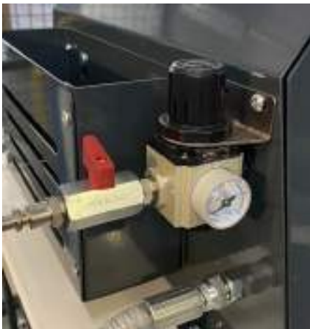
SUPPLY UNIT , consisting of interchangeable quick coupling for connection to the pneumatic network, tap valve, pressure regulator and pressure gauge
