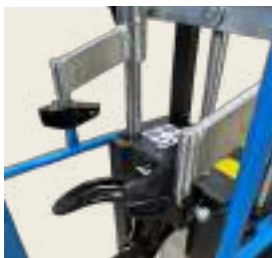
THE TWO AUTO LEVELING UPPER ARMS work easily both on conical and misaligned springs.
