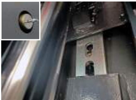
WEDGE RELEASED THROUGH ELECTROMAGNET
