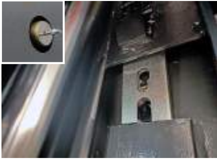
WEDGE RELEASED THROUGH ELECTROMAGNET
