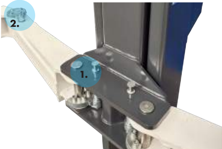
ARM SAFETY LOCKING with automatic engagement and automatic release when the arm reaches the floor
