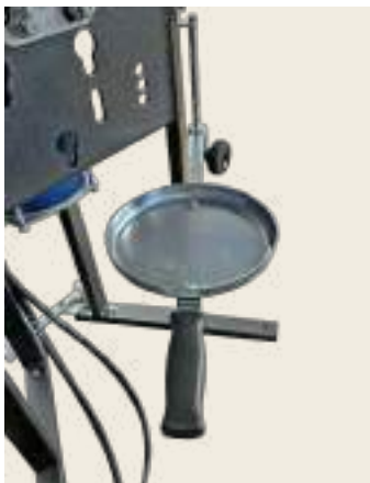
SUPPORT FOR THE HYDRAULIC PART OF THE SHOCK ABSORBER keeps the absorber in position during installation.
